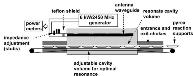
**Figure 2.** Schematic drawing of a multimode tunnel microwave reactor with conveyor and open Pyrex support developed by Esveld and co-workers.
