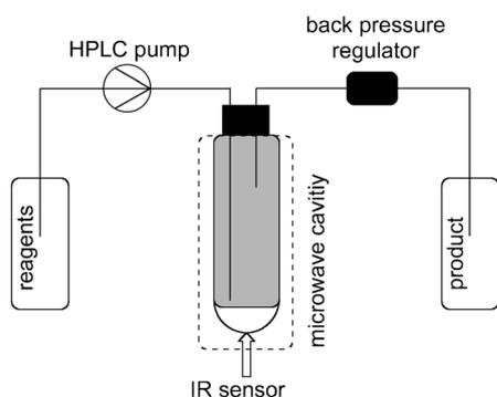
**Figure 4.** Schematic drawing of a microwave synthesizer with a glass-tube reactor.
