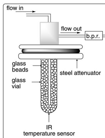
**Scheme 10.** Microwave-assisted continuous Biginelli reaction and rearrangement (*top*), schematic drawing of microwave cavity and flow cell employed (*bottom*).
