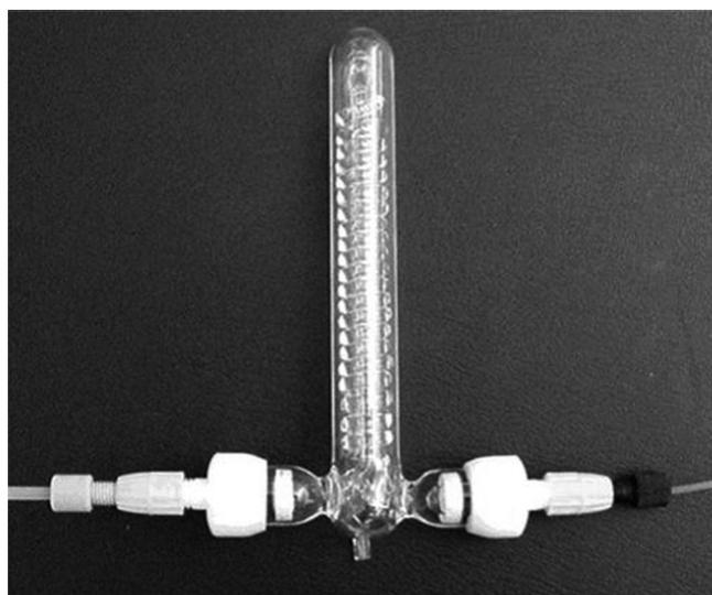
**Figure 3.** Microwave borosilicate glass coil used by Wilson et al. as well as Ley et al. (from ref.<sup>[28]</sup>).
