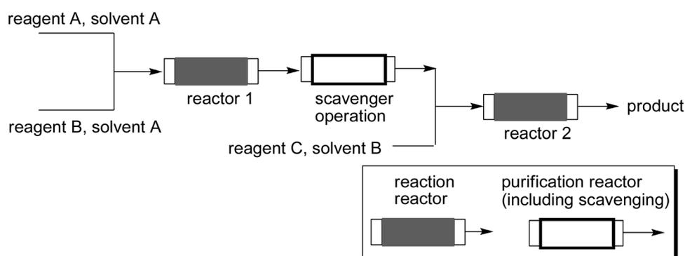
**Scheme 32.** Principal multistep continuous-flow set-up and roles of flow devices as reactors and purification devices (for clarity reasons, two types of graphical presentations are used in the following schemes, one showing a synthesis the other one representing a purification reactor).
