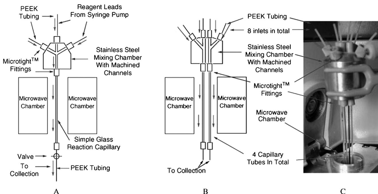
**Figure 5.** Schematic drawing of Organ's capillary reactors inside a microwave cavity (from ref.<sup>[40]</sup>).
