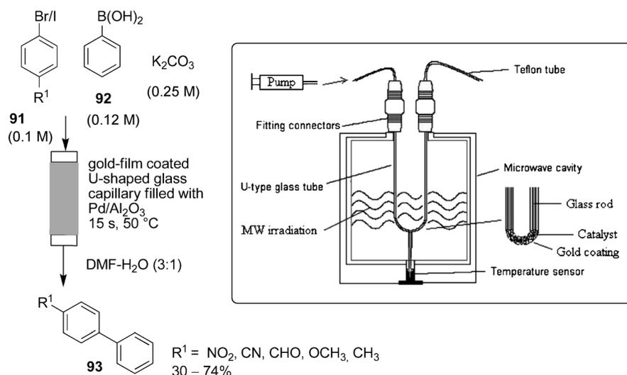
**Scheme 16.** Schematic drawing of Fletcher's and Haswell's gold-coated capillary microwave flow reactor and Suzuki–Miyaura cross coupling reaction (from ref.<sup>[45]</sup>).
