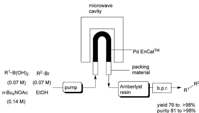
**Figure 6.** Schematic drawing of the flow set-up used by Ley and co-workers.
