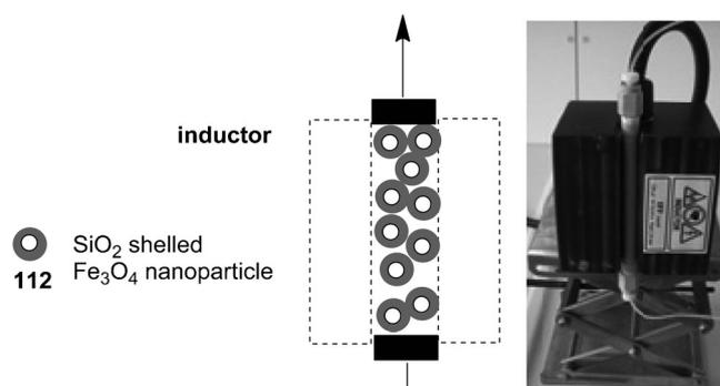
**Figure 7.** Flow reactor filled with magnetic nanoparticles (*left*) and PEEK reactor encased with an inductor (*right*).
